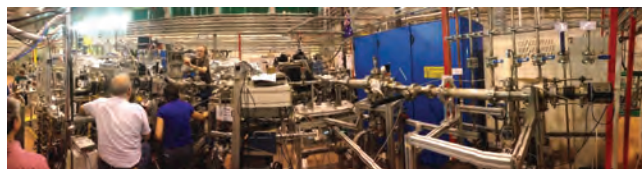
Figure 4: Set-up of the experiment to detect spontaneously triggered stimulated emission from doubly excited states of He at the LDM beamline of the free-electron laser facility FERMI in Trieste.
