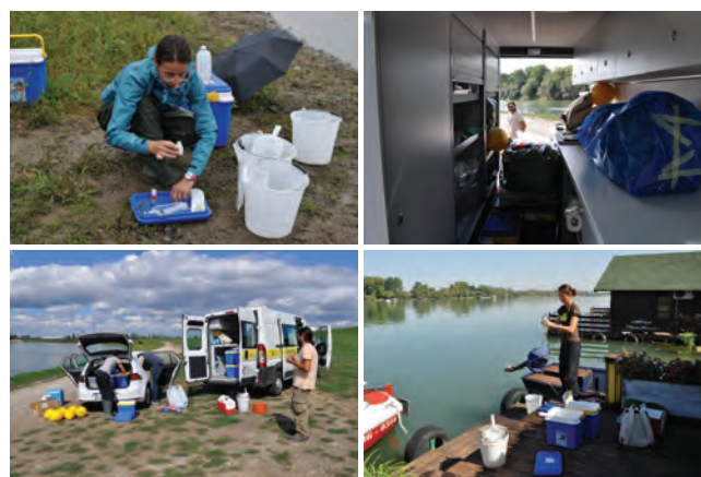
Figure 5: As part of the EU project GLOBAQUA in September 2015, co-workers from the Department of Environmental Sciences performed the sampling of water, biota and sediments of the Sava River from Mojstrana to Belgrade. The sampling was performed with the use of the new, fully equipped van of the Ecological Mobile Unit Laboratory.
