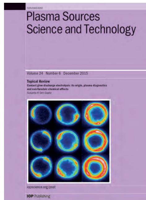
Figure 1: This figure from the paper of our coworker Dr Matjaž Panjan was selected as a cover image for the journal Plasma Sources Science and Technology. It shows plasma structures in DC magnetron sputtering, recorded using a high-speed camera (exposure time 500 ns).
