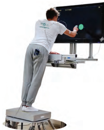
Figure 5: Experimental setup for investigating mechanisms of human motor control in contact with the environment.
