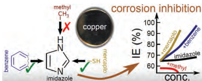
Figure 2: Effect of derivatives of imidazole on the efficiency of corrosion inhibition on copper in a chloride solution.
