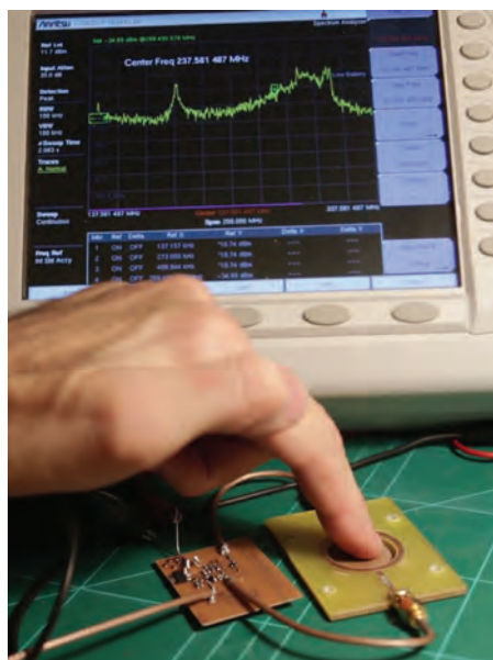
Figure 2: Bioimpedance sensor developed at the department in collaboration with the Hyb company.
