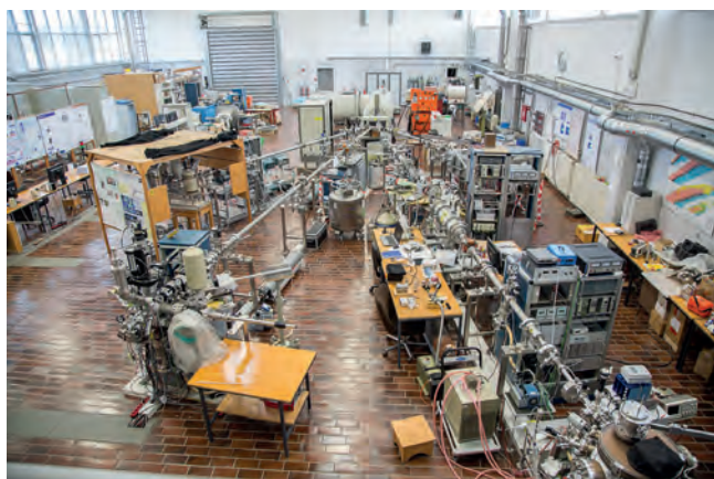
Figure 6: 2 MV tandem accelerator of the Jožef Stefan Institute with four beamlines (Foto M. Verč).
