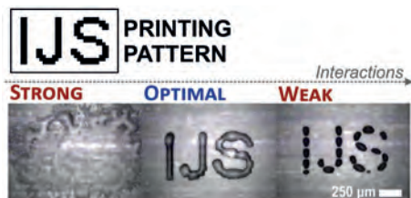
Figure 7: The impact of the ink-substrate interactions on the morphology and definition of the printed pattern. The indium-zinc oxide (IZO) ink (prepared by dissolving \text{In}(\text{NO}_3)_3 and \text{Zn}(\text{NO}_3)_2 in a solvent mixture of 2-methoxyethanol and 1,3-propanediol in a 45:55 volume ratio) spreads completely on the bare glass due to strong interactions (left). By implementing a PMMA layer, the interactions become weak and the pattern breaks into individual droplets (right). A precise adjustment of the interactions between the ink and the substrate by a partial decomposition of the polymeric layer enables printing with a high resolution (middle). The results of the study were published in A. Matavž, V. Bobnar, B. Malič. Tailoring ink-substrate interactions via thin polymeric layers for high-resolution printing. Langmuir 33, (2017), 11893.
