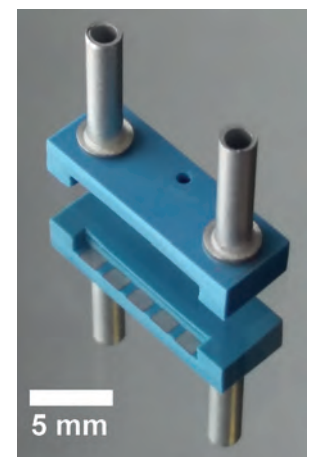
Figure 5: Fluidic channel in LTCC structure with integrated pressure sensor.
