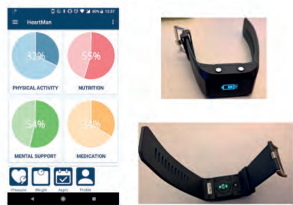
Figure 4: HeartMan mobile application, which helps patients with heart failure manage their disease, and the sensing wristband that collects the patients' physiological signals for the application.
