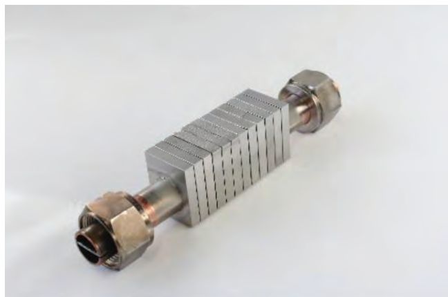
Figure 5: Composite monoblocks joined to a CuCrZr cooling tube and subjected to HHF tests in an actively cooled divertor model
