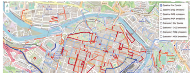
Figure 4: This visualization exemplifies a simulated traffic scenario, forecasting the consequences of closing Bilbao's central square to traffic. This tool is one among numerous resources offered by the platform established during the URBANITE project.
