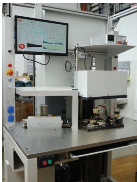
Figure 8: Semi-automatic end-of-line quality inspection system, type 714, for the Domel company
