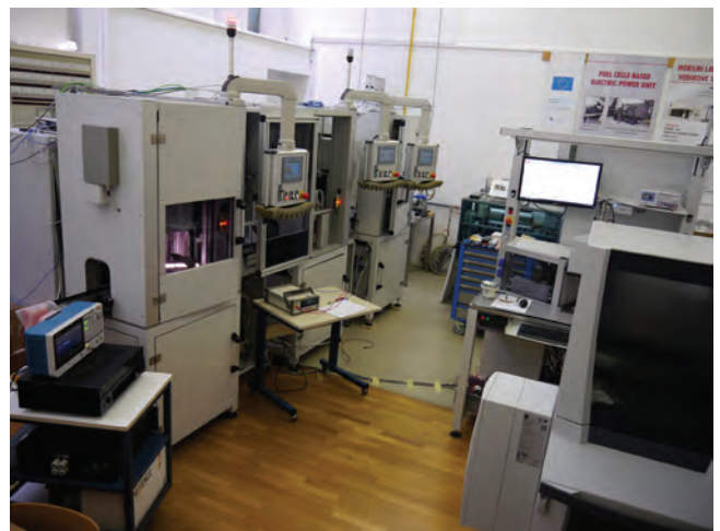
Figure 7: Fully automatic end-of-line quality inspection system, type ML16, for the Domel company (development and fabrication at the JSI)
