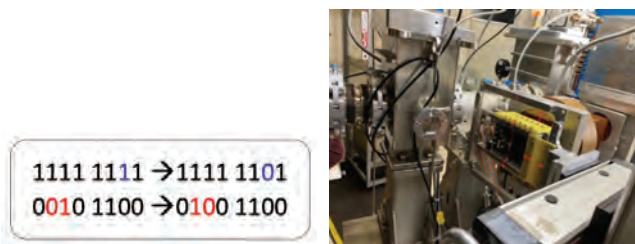
Figure 3: During the tests with the accelerator at the Paul Scherrer Institute (PSI) in Switzerland, where we searched for the so-called Single Event Effect-e (SEE), two such events were recorded by the Calypso ASIC (left image). The right picture shows the set-up of the experiment where we used a laser to align the electronic circuit in the proton beam.
