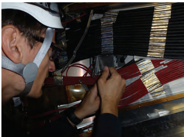
Figure 2: Installation of Diamond beam monitor (DBM) on the support structure of pixel detector. It will provide complementary luminosity measurement to the BCM
