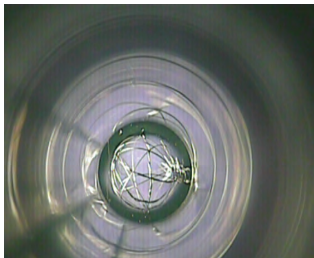
Figure 1: An inverted fire-ball in the magnetized plasma of the Linear magnetized plasma device in the Laboratory for Plasma Physics in the Reactor Physics Department of the JSI. The grid of the wired-ball is at a higher potential than the surrounding plasma and together with the inter-grid spaces forms an equipotential surface. The electrons in the surrounding plasma see it as a virtual anode, towards which they accelerate and with additional ionization form a new plasma on the inside.
