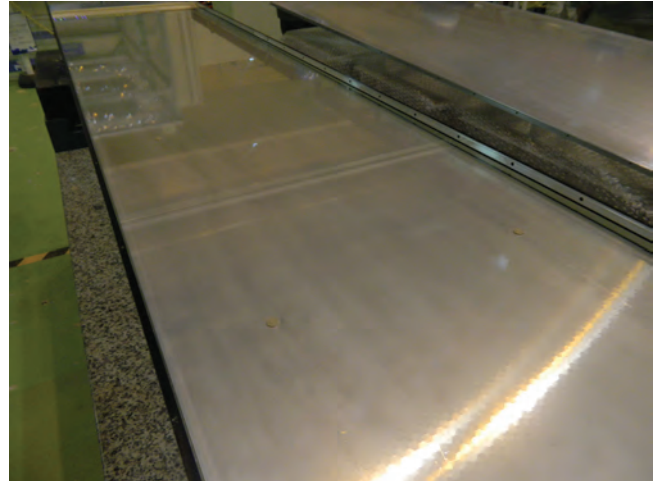
Figure 4: Preparation of quartz modules for charged particle identification through the detection of the Cherenkov light in BELLE spectrometer
