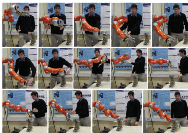
Figure 1: Human-robot cooperative task execution.
