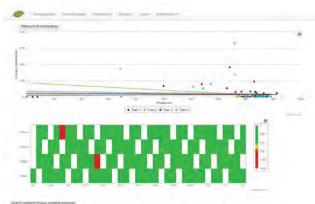
Figure 3: LifeSaver representation of the energy consumption per day using the operator's working shift as a context variable (contour diagram)
