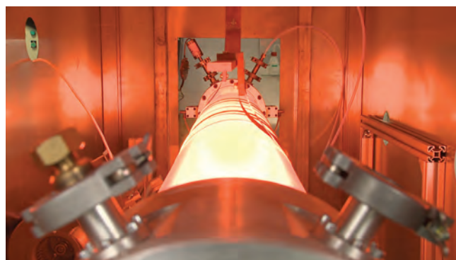
Figure 1: Glowing nitrogen plasma emits radiation at different wavelengths, peaking in the orange part of the optical spectrum
