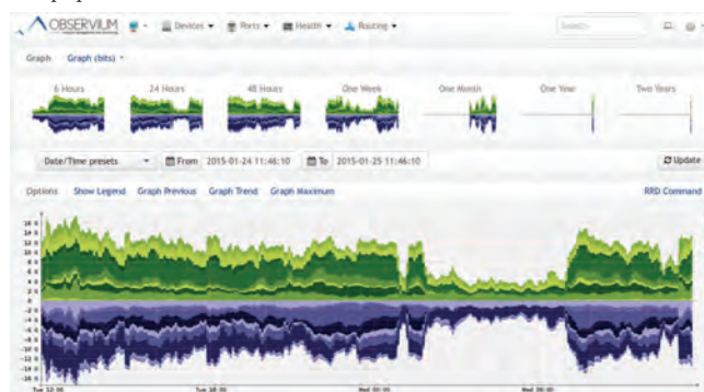
Figure 3: Observium displaying data transfer rates on one of the new routers in the core JSI network.
