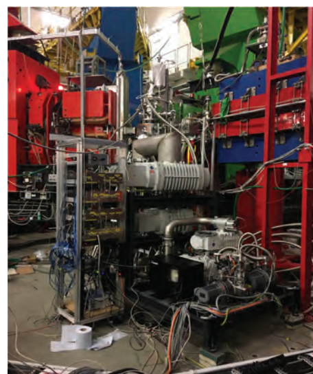
Figure 1: New hypersonic jet target at the A1 experimental hall in Mainz Microtron (MAMI), built for an upcoming series of high-precision nuclear experiments with electrons on various nuclear targets.
