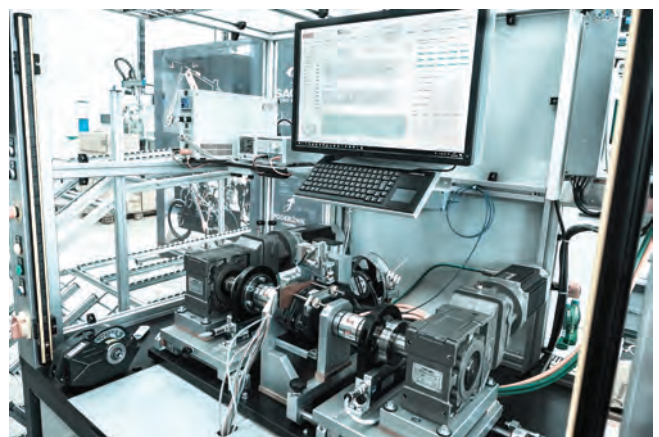
Figure 5: Diagnostic System for End-Of-Line Quality Assessment of the Pedelec Electric Bike Drives
