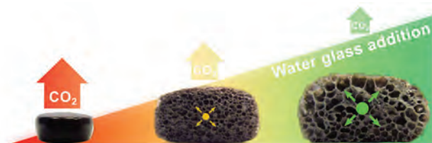
Figure 6: Higher addition of water glass allows the same expansions to be achieved at lower temperatures, which has a favourable effect on the energy complexity of production.
