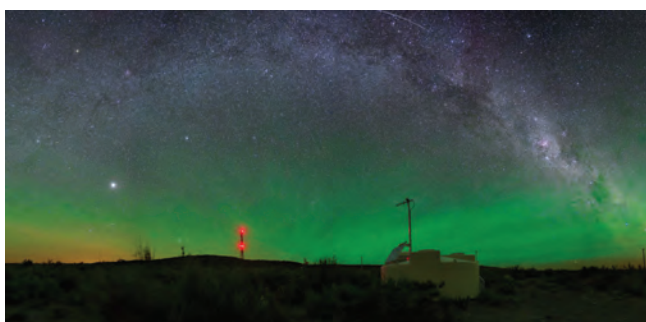
Figure 6: Figure shows one of 1600 ground Cherenkov detectors at the Pierre Auger Observatory. In background communication tower for DAQ data transfer. Detector network covers an area of 3000 \text{ km}^2 .
