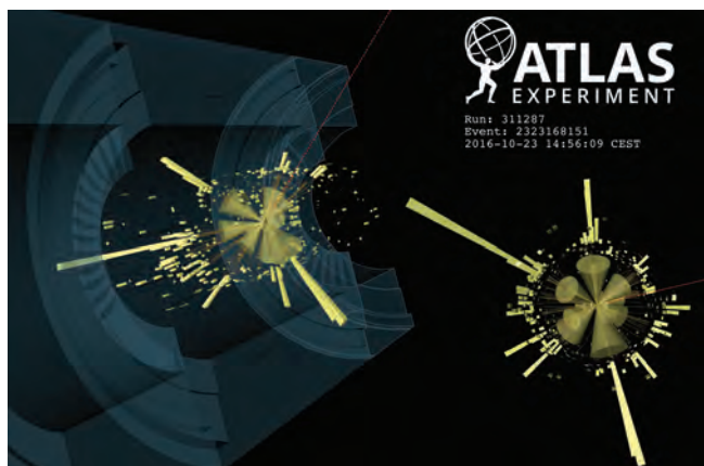
Figure 1: Event display visualisation of the highest jet multiplicity event selected in signal regions targeting long cascade decays of pair-produced gluinos. This event was recorded by ATLAS on 23 October 2016, and contains 16 jets, illustrated by cones. Yellow blocks represent the calorimeter energy measured in noise-suppressed clusters.
