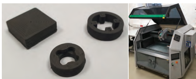
Figure 2: 3D printed magnets produced by fused-filament fabrication. The particles were orientated during the printing with an external magnetic field.
