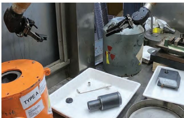
Figure 10: Manipulation of the new ^{137}\text{Cs} source in the hot cell of JSI. In 2020, we installed the new ^{137}\text{Cs} and ^{60}\text{Co} sources in the irradiator of the National laboratory for dosimetry standards, providing a gamma irradiation field for the national etalon of ionizing radiation.
