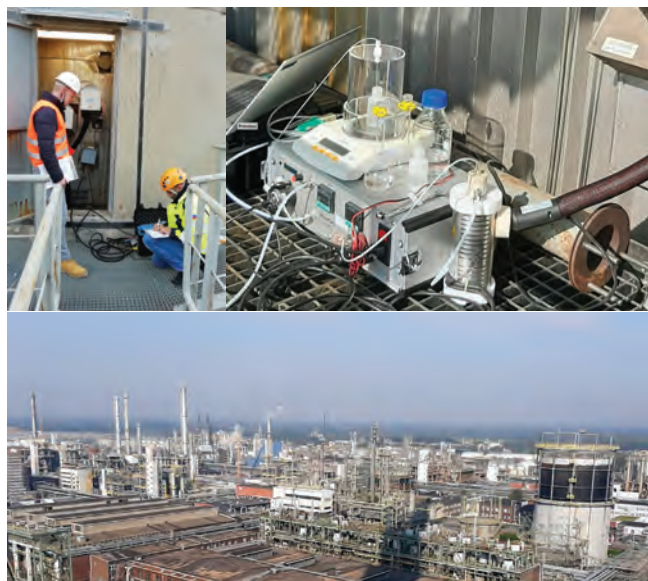
Figure 1: Calibration of mercury-emission measurements with traceable calibration methods developed in the MercOx project was used in field measurements at Salonit Anhovo (above) and at the thermal power plant in Marl, Germany (below)
