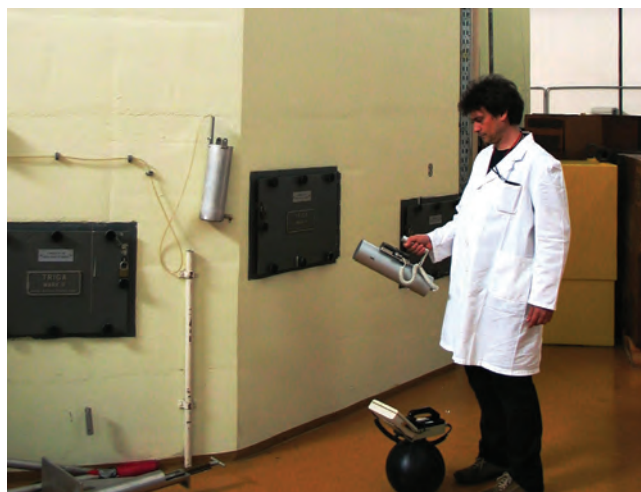
Figure 1: Dose-rate measurements near the experimental channels in the hall of the TRIGA MARK II reactor
