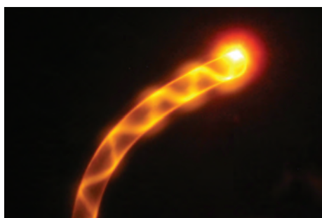
Figure 14: Smectic-A liquid crystal spontaneously forms optical fibres that are excellent waveguides and laser emitters.
