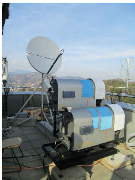
Figure 2: Alphasat satellite receiver, developed at the JSI and installed in collaboration with the Joanneum Research Institute on the Hilmwarte tower in Graz, Austria.
