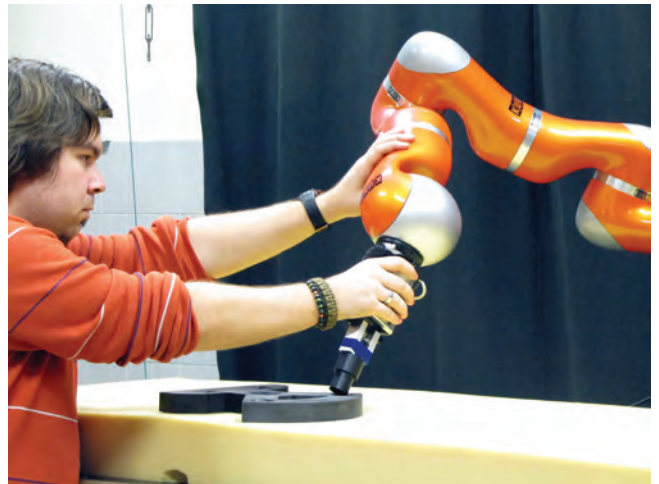
Figure 4: An imitation learning system that can take into account forces and torques arising in tasks that involve contact with the environment.
