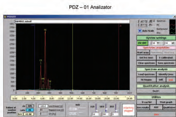
Figure 7: Interface of PDZ-01 XRF analyser, developed at the department (P. Kump and Z. Rupnik).
