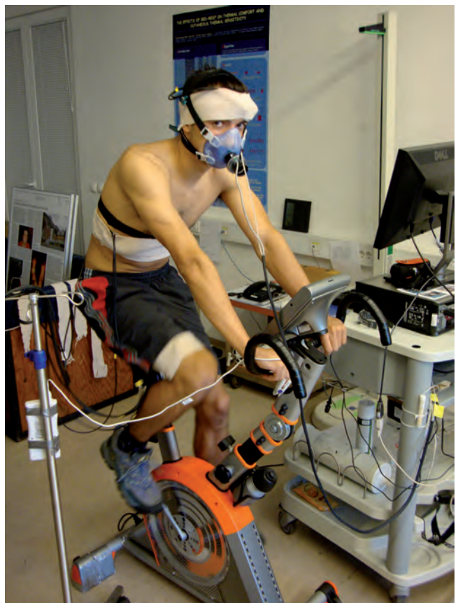
Figure 5: A subject during a maximal incremental exercise test on the cycle-ergometer, while oxygen consumption and cerebral and muscle oxygenation are measured.
