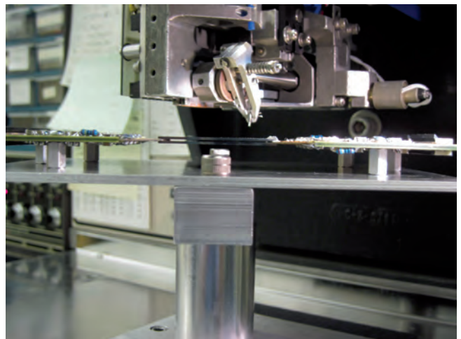
Figure 5: Assembly of a silicon detector module for the PET probe.
