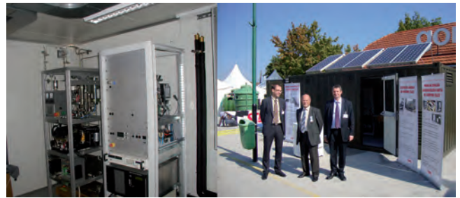
Figure 4: TESTLAB subunits: electrolyser, methanol reformer, fuel cells (left); Presentation of the mobile experimental laboratory TESTLAB at the event SOBRA 2010, G. Radgona, Slovenia (right)
