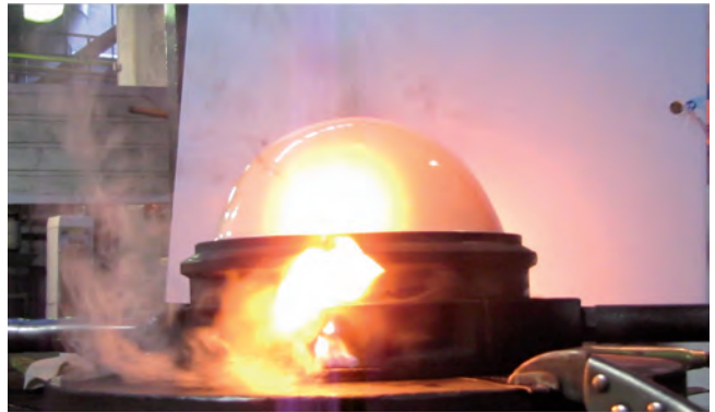
Figure 4: Computer-controlled shaping operation of a glass melted semi-product.
