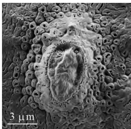
Figure 17: Nanoparticle from the ash erupted from volcano Eyjafjallajökull and brought by air flow to Kravac in Slovenia. It contained metal sulphides and fluorides, which at a presence of humidity caused its corrosion. The image was taken by scanning electron microscope at national Institute of Chemistry. Author: G. Kapun
