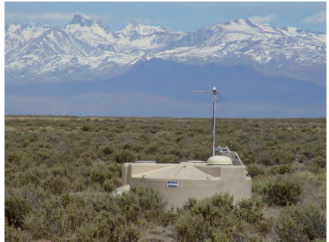
Figure 4: Čerenkov detectors placed in the so-called Ground Array. More than 1600 such detectors measure high-energy particles through their interaction with water
