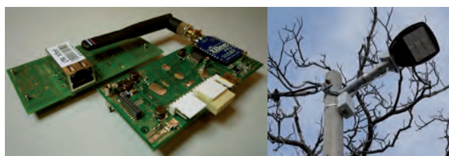
Figure 3: Versatile sensor node (VSN) for the research and development of semantic sensor networks (left) and its deployment in a street-lighting testbed (right)
