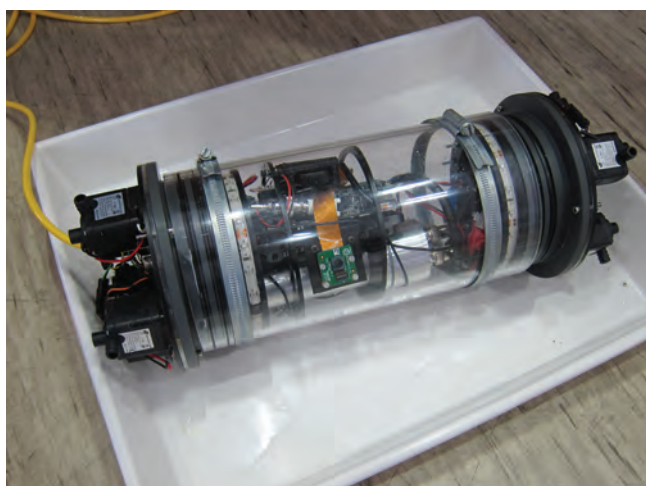
Figure 4: Underwater ROV that will investigate the interior of the damaged reactor in Fukushima.
