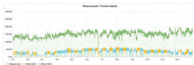
Figure 5: Power consumption of the JSI computer centre Teslova reflects how much the facility is used. There is a short drop at the end of June due to an unscheduled cooling-system maintenance caused by power fluctuation. The graph shows higher efficiency of the cooling system in the winter months, when the air is sufficiently cool to use free cooling.
