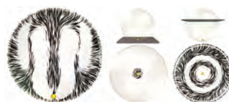
Figure 14: A layered structure in a chiral nematic droplet with cylindrical symmetry and a single point defect.
