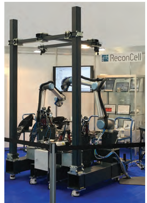
Figure 1: Reconfigurable robot workcell at Automatica 2018 in Munich, Germany
