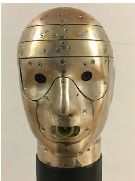
Figure 6: Sweating thermal head manikin
