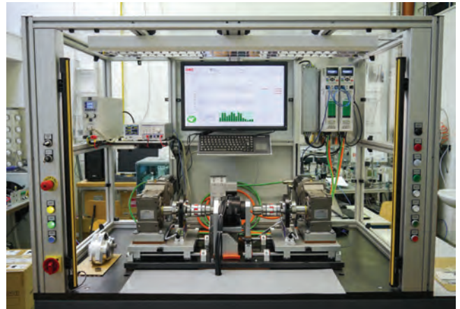
Figure 4: Diagnostic system for End-of-line control of electric drives for bicycles of the Pedelec type (Pedal Electric Cycle)
