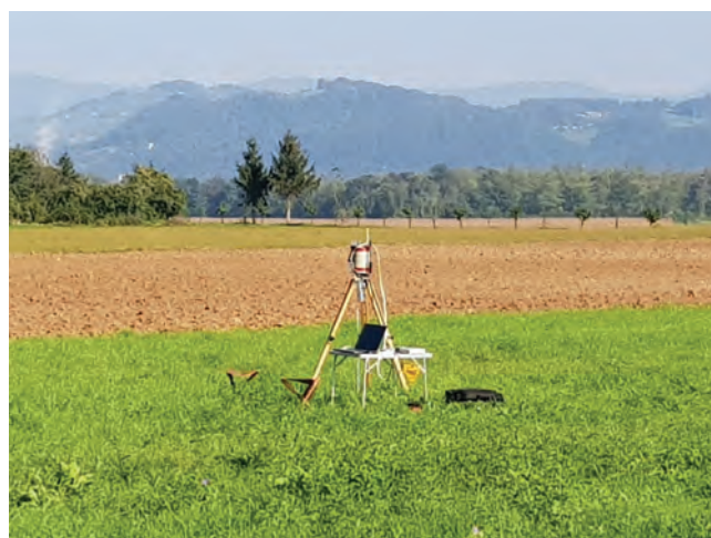
Figure 1: Measurements of gamma radioactivity in situ with a high-purity germanium spectrometer within the environmental monitoring of the radioactivity in the environment
