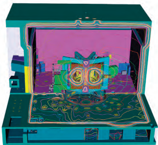
Figure 3: Visualization of the full 3D model of the JET tokamak used for calculations of streaming experiments. The contour plot shows the neutron flux originating from DT plasma contained in the vacuum vessel simulated using a discrete ordinates deterministic neutron transport code.
