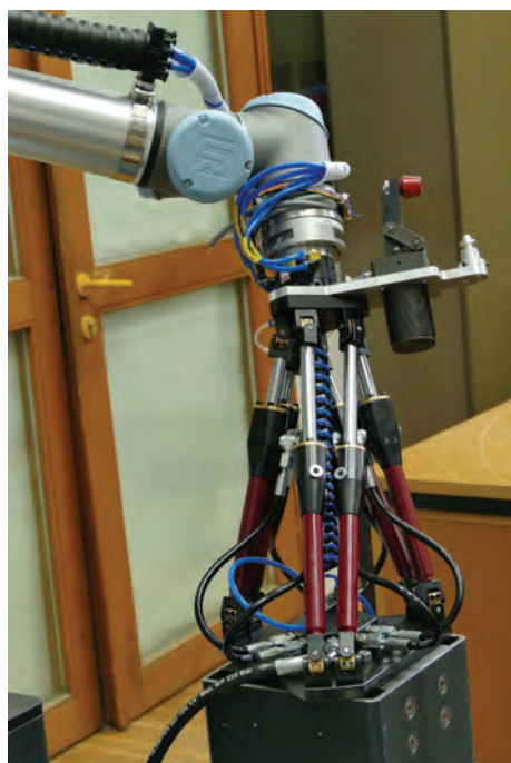
Figure 2: Passive fixture reconfigured by a robot
