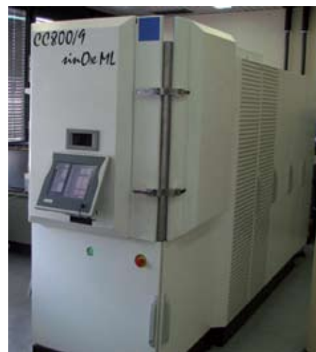
Figure 1: New apparatus for the deposition of hard coatings, CemeCon CC800/9 sinOx
