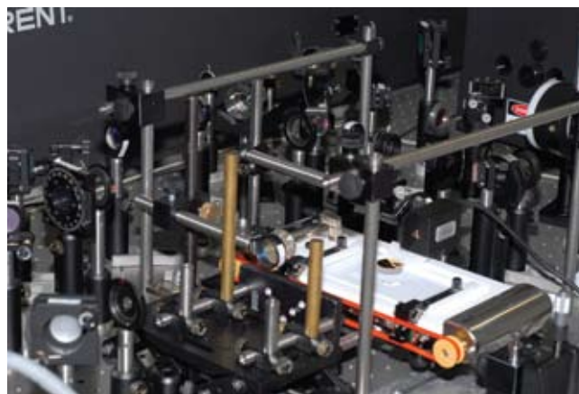
Figure 4: Experimental setup for non-linear optical spectroscopy (IR-VIS SFG) of Langmuir films of biomolecules on the surface of water.
