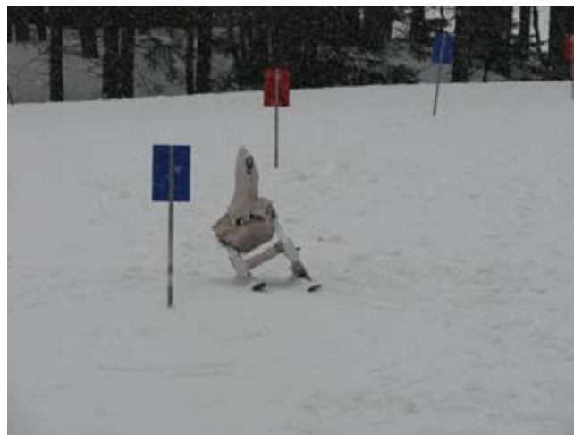
Figure 5: Robot skier mechanism on a ski slope skiing between gates
