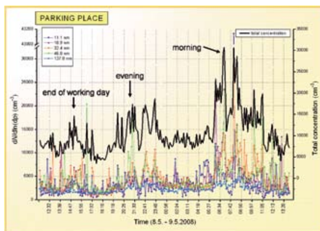
Figure 3. Concentrations and size distribution of nano-aerosols at a parking place near heavy traffic.
