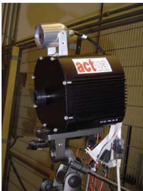
Figure 2: Arflex FP6 project result: embedded robot-vision system (smart camera)
