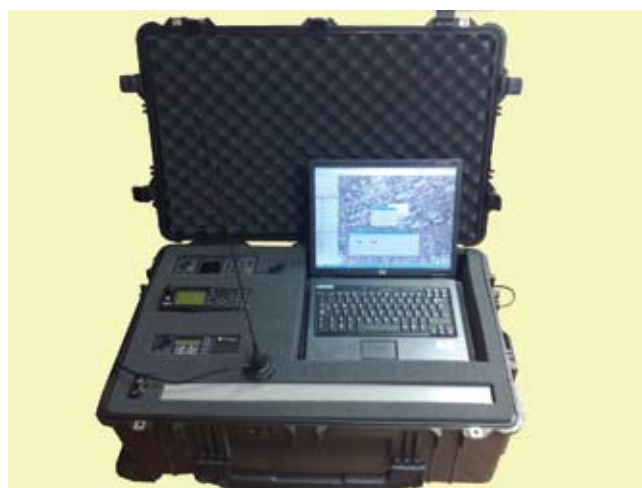
Figure 1: Mobile integrated device for the measurement, recording, presentation and analysis of a signal level in mobile radio systems for emergency communications ZARE, ZARE+, DMR and TETRA
