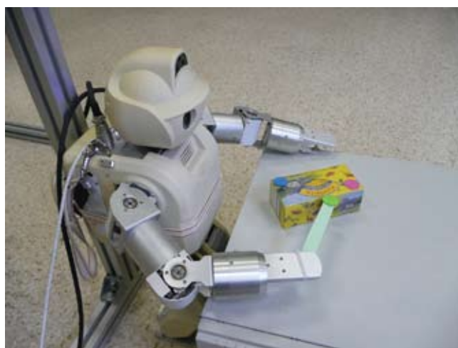
Figure 1: Humanoid robot HOAP using humanoid vision for autonomous learning of object pushing
