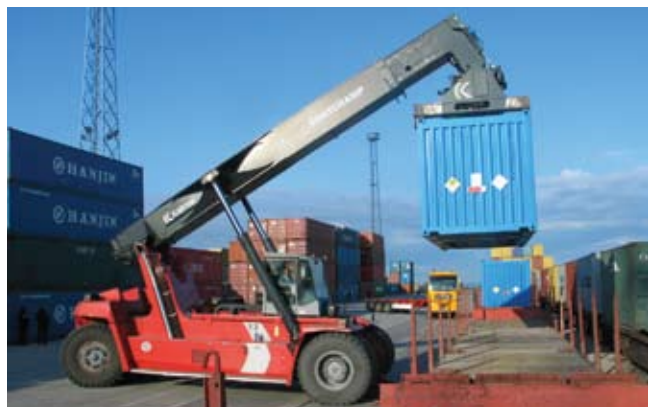
Figure 2 : Handling of transport containers containing spent fuel
