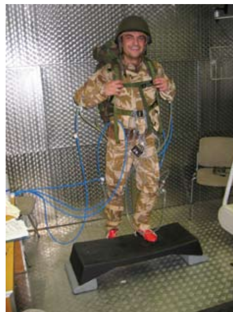
Figure 4: Evaluation of military equipment for desert conditions in a climatic chamber
