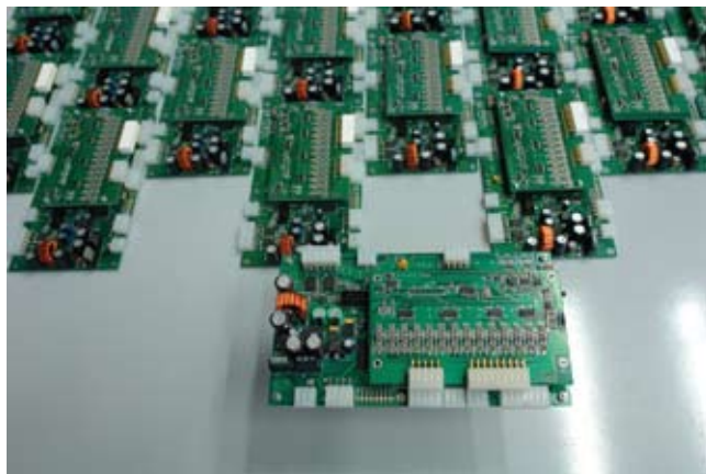
Figure 4: SmartModule - an Air Delivery Control System intended for the control of air flow in the fuel-cell and natural-gas reformer based on a co-generation heating/power supply system
