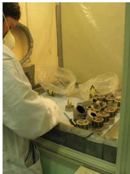
Figure 5: Disassembling of smoke detectors with americium-241, performed as part of the project “Improvement of the management of institutional radioactive waste in Slovenia”.
