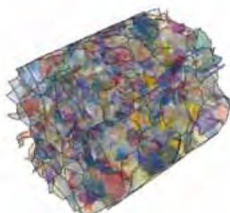
Figure 2: Reconstruction of grain boundaries in AISI 304 stainless steel.
