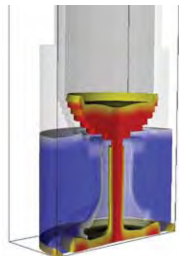
Figure 1: Simulation of the fuel-coolant interaction during reactor-core melt release from a failed reactor pressure vessel.
