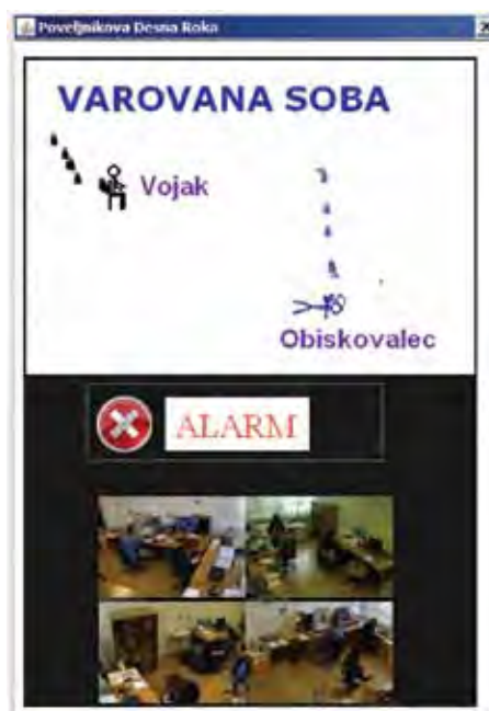
Figure 1: The control panel of the intelligent security system ("PDR" project), where the situation in the surveilled rooms is presented with a live picture, a symbolic-graphical and textual description.
