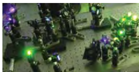
Figure 2: Non-collinear optical parametric amplifier for the generation of sub-20 fs pulses
