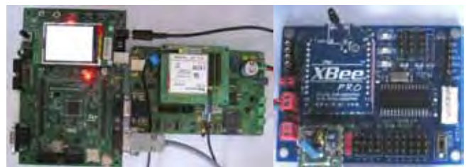
Figure 5: Sensor (left) and gateway (right) nodes in a two-tiered wireless-sensor network
