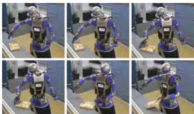
Figure 2: The humanoid robot is pushing an object in order to support grasping. The pushing action has been learned autonomously by exploration of the robot's environment without prior knowledge. This work has been done in collaboration with the Karlsruhe Institute of Technology, Germany.
