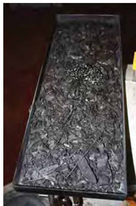
Figure 5: The picture shows the carbon-rich residue after wooden biomass pyrolysis, which enables the production of pure fuels for different purposes, including applications in fuel cells.
