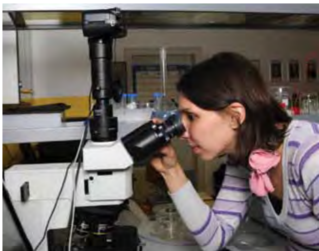
Figure 2: The changes at a metal's surface caused by a corrosion attack are often analysed using an optical microscope.
