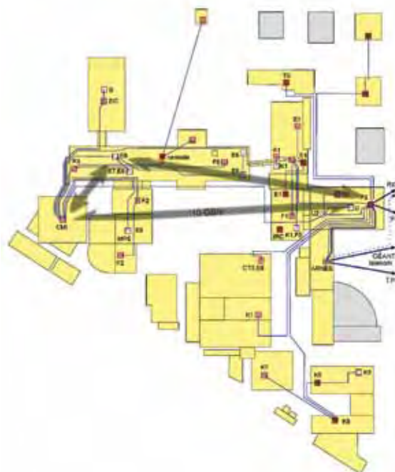
Figure 2: Layout of JSI communication network
