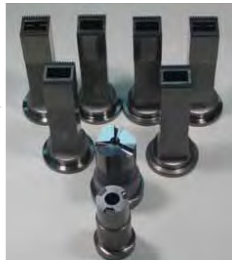
Figure 5: Tool for metal powder compaction protected by the "black coating"; in the Unior company; program Sinter; it is used in the production of several automotive components
