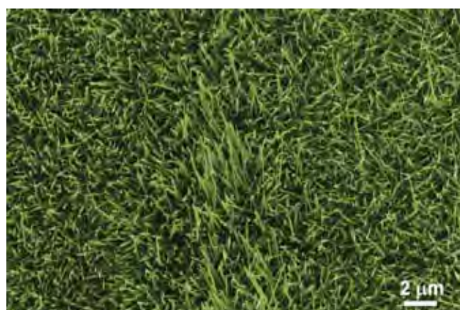
Figure 2: Nano meadow: \text{TiO}_2\text{-Al}_2\text{O}_3 crystals grown from the Ti6Al4V alloy during thermal treatment in Ar 99.99
