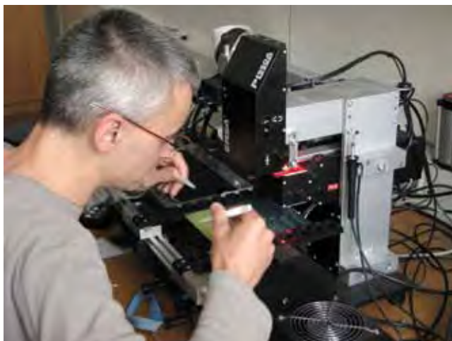
Figure 5: Assembly of the detector module using BGA (Ball Grid Array) technology
