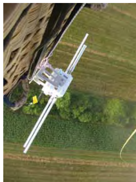
Figure 1: WLAN mesh router mounted on a hot-air balloon for radio-wave propagation measurements in emergency situations
