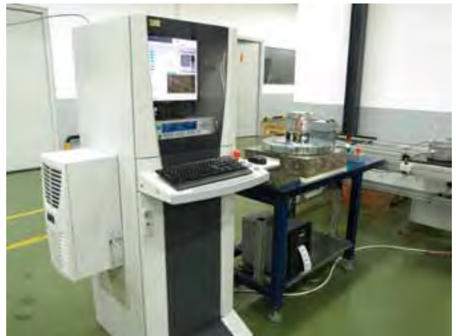
Figure 5: Diagnostic system for electronically commutated motors.
