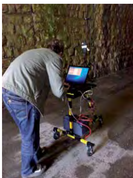
Figure 3: Radio-wave propagation measurements in a tunnel
