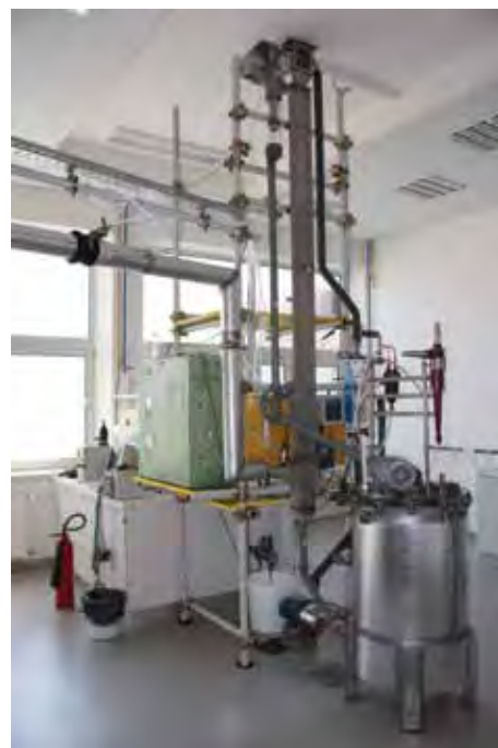
Figure 4: Laboratory device for waste-gases desulphurization. The reconstructed device will allow the optimisation of the desulphurization process. It will also be used for the laboratory research of mercury removal from waste gases.
