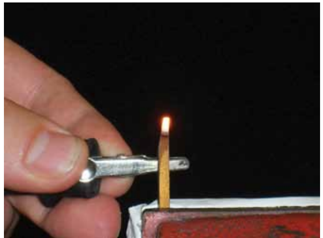
Figure 4: The ceramic heater prepared from a silicon-nitride-based composite with dispersed conductive particles
