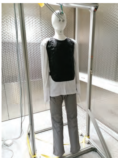
Figure 7: Manikin for testing protective garments
