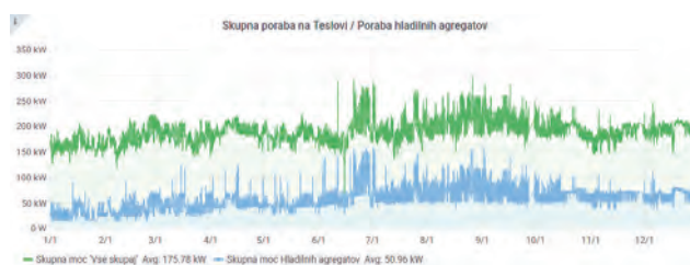
Figure 4: Power consumption of the JSI computer centre Teslova reflects how intensively the facility hosting our HPC systems is used. The graph shows higher efficiency of the cooling system in winter months, when we can use free cooling, and increased consumption in the second half of the year, when the power requirements forced us to start using both cooling systems in parallel.
