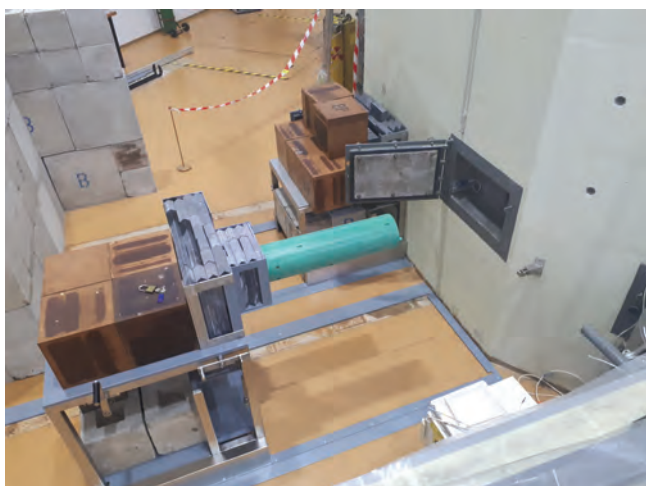
Figure 5: Last year, beam port No. 5 was modified for the purpose of irradiating large fission chambers. The facility is used by Rolls Royce Civil Nuclear S.A.S.
