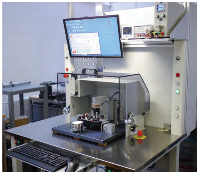
Figure 5: Diagnostic system for end-of-line control of electromotor for bicycle electric drive
