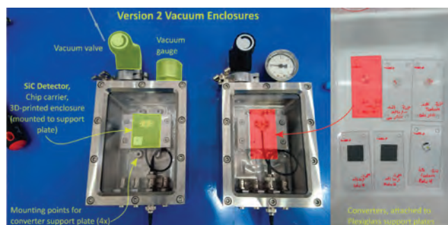
Figure 1: Prototype neutron detectors based on silicon carbide (SiC), developed in the E-SiCure project and tested in the JSI TRIGA reactor. The detectors operate in a vacuum environment and consist of SiC Schottky barrier diodes and neutron to charged particle converting films of ^{10}\text{B}^{14}\text{C} or ^6\text{LiF} , around 2 \mu\text{m} in thickness, deposited onto aluminium substrate.
