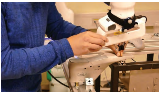
Figure 3: Robot programming by human demonstration of shoe finishing operation
