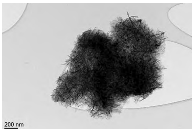
Figure 8: TEM image of the Ru nanoparticles-decorated magnetic alumina catalyst (Gyergyek S., K8, JEM 2100).
