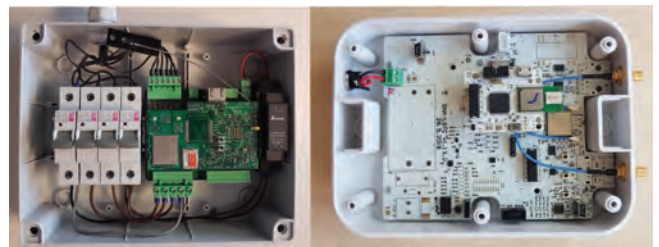
Figure 3: SAAM system components: PMU in additional external housing and eGW with integrated UWB transceiver
