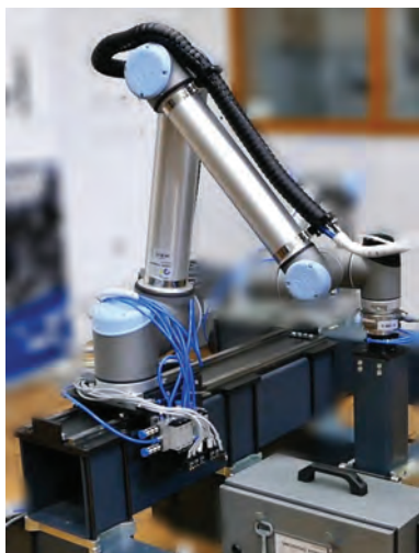
Figure 2: Passive linear rail developed in the ReconCell project to support workcell reconfiguration
